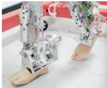
Figure 2.4. The 2-DOF ankle-foot system based on the compliant mechanism [20].
